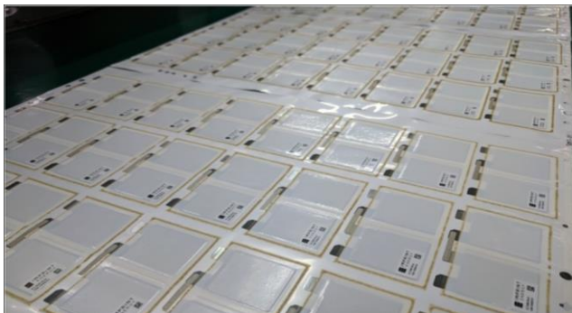
printed batteries (source: Imprint Energy))
